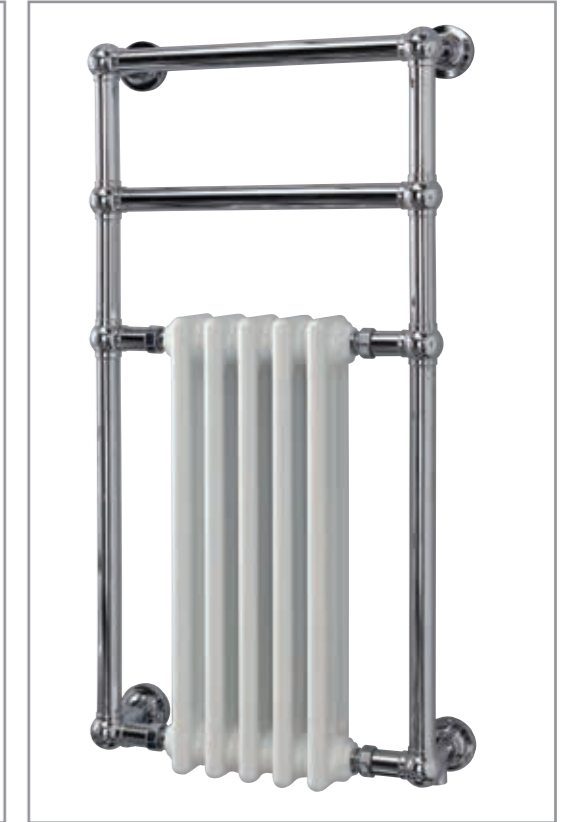
SSPINSB4CR • Radiatore a muro con inserto in ghisa bianco mm.975x475 DT60° 582Kcal/h - 675 Watt Radiateur mural avec insert en fonte blanche mm.975x475 DT60° 582Kcal/h - 675 Watt Wall mounted radiator with white cast iron insert mm.975x475 DT60° 582Kcal/h - 675 Watt
