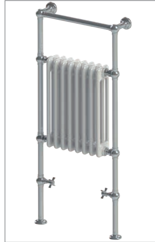
SSPVB3CR • Radiatore a pavimento cromo con inserto in ghisa mm.1185x545 DT60° Kcal/h 623,6 - Watt 723 Radiateur de sol chromé avec insert en fonte 1185x545mm. DT60° Kcal/h 623,6 - Watt 723 Floor mounted radiator chrome with cast iron insert 1185x545mm. DT60° Kcal/h 623,6 - Watt 723
